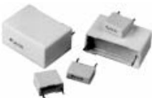
Type 171 radial leaded, box, metallized polypropylene capacitors are available in five pitch sizes and have a flame retardant case and epoxy encapsulant that meets UL94V-0. The Type 171 is an excellent choice for applications requiring low dielectric losses, high insulation resistance in an AC or DC environment. The polypropylene dielectric gives this capacitor excellent pulse rise time (dv/dt) performance.
