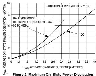
Figure 2. Maximum On-State Power Dissipation
