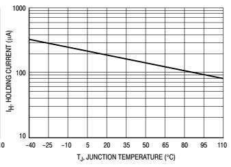
Figure 4. Typical Holding Current versus **Junction Temperature**
