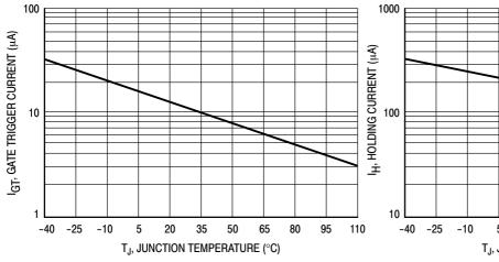
Figure 3. Typical Gate Trigger Current versus Junction Temperature
