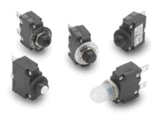
Rating: 3 to 20A, 125-250VAC, 32VDC Approvals: *UL, CUL, TUV, CE UL1500/ISO8846 for ignition protection/marine* Dielectric Strength: 2500 VAC/ 1 minute Interrupting capacity: 2500 amps Resettable overload capacity: 10x rated current Insulation Resistance: 100M ohms
