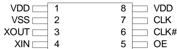
Figure 1. Pin Diagram - 8-Pin TSSOP
