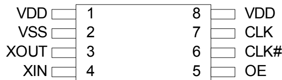
Figure 1. Pin Diagram - 8-Pin TSSOP
