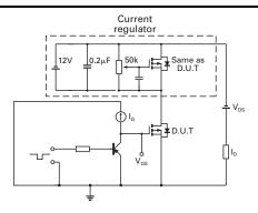
Gate charge test circuit
