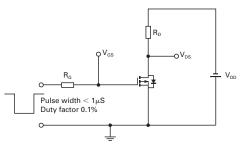
Switching time test circuit
