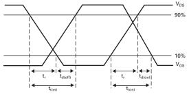
Switching time waveforms
