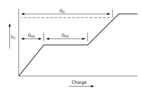
Basic gate charge waveform
