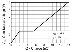
Gate-Source Voltage v Gate Charge
