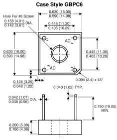
Polarity shown on side of case: Positive lead by beveled corner
