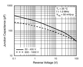
Figure 5. Typical Junction Capacitance Per Diode
