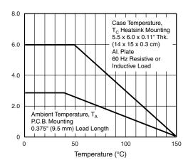
Figure 1. Derating Curve Output Rectified Current
