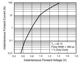
Figure 3. Typical Forward Characteristics Per Diode
