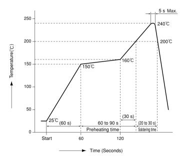
Applicable Conditions Reflow system: IR reflow Solder type: Cream type 63 Sn/37 Pb (Flux component 9 wt%) Test board: Glass epoxy 85 x 60 x 1 mm Metal mask thickness: 0.15 mm
