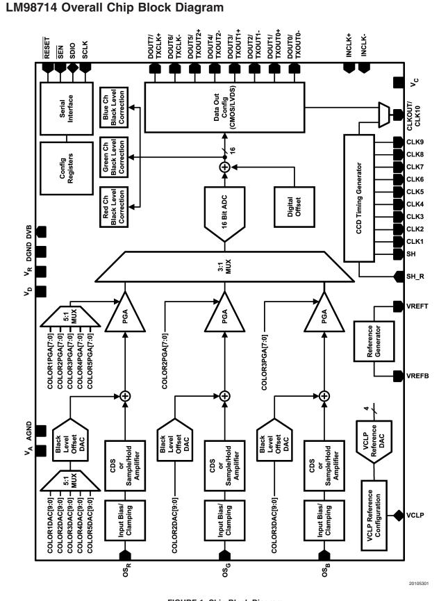
FIGURE 1. Chip Block Diagram
