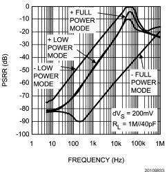
**Typical Performance Characteristics** Unless otherwise specified,  $V^+ = 5V$ ,  $T_A = 25^{\circ}C$ ,  $PS = V^+$  for Full Power Mode,  $PS = V^-$  for Low Power Mode. (Continued)
