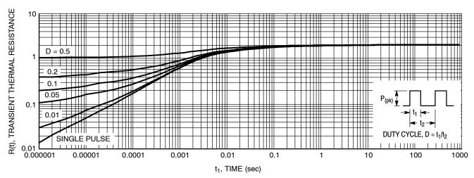
Figure 9. Thermal Response Junction-to-Case for MBR20H100CT and MBRB20H100CT
