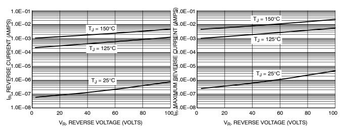
**Figure 3. Typical Reverse Current**
