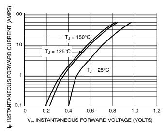
Figure 1. Typical Forward Voltage
