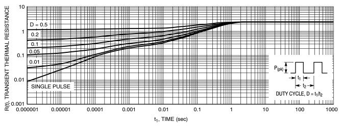
Figure 10. Thermal Response Junction-to-Case for MBRF20H100CT
