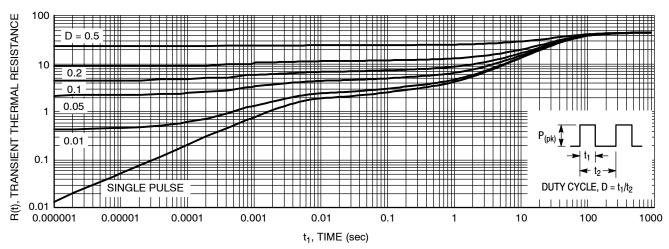
Figure 8. Thermal Response Junction-to-Ambient for MBR20H100CT and MBRB20H100CT
