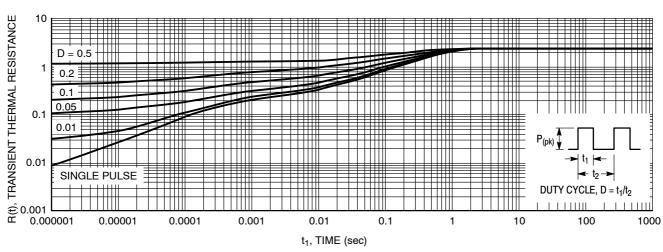
Figure 10. Thermal Response Junction-to-Case for MBRF30H60CTG
