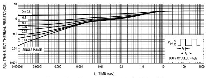
Figure 11. Thermal Response Junction-to-Case for MBRF2045CT
