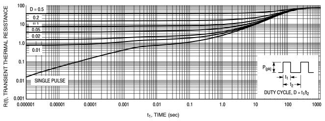
Figure 10. Thermal Response Junction-to-Ambient for MBRF2045CT
