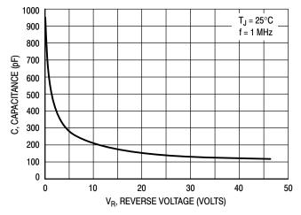
Figure 12. Typical Capacitance
