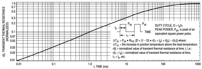
Figure 9. Thermal Response for MBR2045CT
