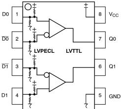
Figure 1. 8-Lead Pinout (Top View)
