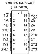
The SN74HC139 device comprises two individual 2-line to 4-line decoders in a single package. The active-low enable  $(\overline{G})$  input can be used as a data line in demultiplexing applications. This decoder/demultiplexer features fully buffered inputs, each of which represents only one normalized load to its driving circuit.
