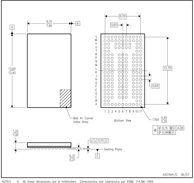
All linear dimensions are in millimeters. Dimensioning and tolerancing per ASME Y14.5M-1994. Α.
