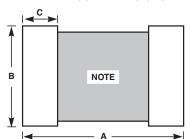
NOTE : Avoid metal runs in this area, parts not recommended for use in applications using Silver Epoxy Paste.
