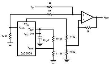
FIGURE 8. Trimming the Offset of a Dual Supply Op Amp Biased at Ground
