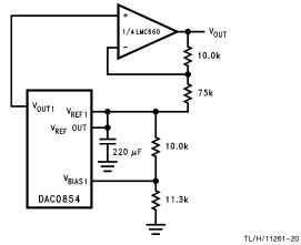
FIGURE 9. Bringing the Output Range Down to Ground
