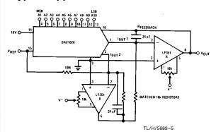
$$\begin{split} V_{OUT} &= -V_{REF} \left( \frac{A1}{2} + \frac{A2}{4} + \bullet \bullet \bullet + \frac{A10}{1024} - \frac{1}{1024} \right) \\ \text{where: AN} &= +1 \text{ if A}_N \text{ input is low} \\ AN &= -1 \text{ if A}_N \text{ input is low} \end{split}$$
