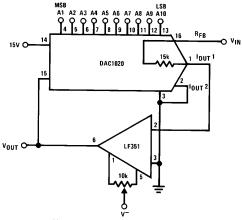
$$V_{OUT} = \frac{-V_{REF}}{\left(\frac{A1}{2} + \frac{A2}{4} + \frac{A3}{8} + \dots \frac{A10}{1024}\right)}$$
