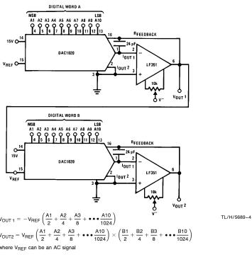
FIGURE 6. Precision Analog-to-Digital Multiplier
