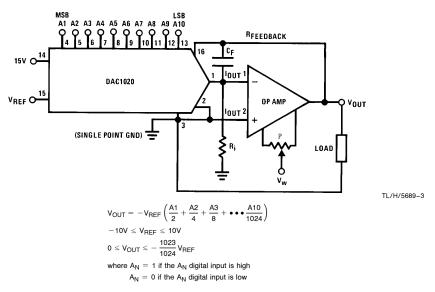
FIGURE 3. Basic Connection: Unipolar or 2-Quadrant Multiplying Configuration (Digital Attenuator)
