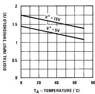
FIGURE 1. Digital Input Threshold vs Ambient Temperature
