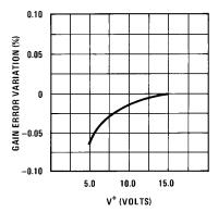
FIGURE 2. Gain Error Variation vs V+
