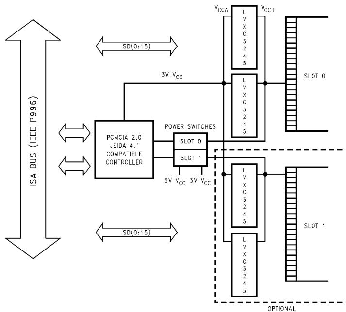
The LVXC3245 is a 24-pin dual supply device well suited for PCMCIA configurable I/O applications. Ideal for low power notebook designs, the LVXC3245 consumes less than 1 mW of quiescent power in all modes of operation. The LVXC3245 meets all PCMCIA I/O voltage requirements at 5V and 3.3V operation. By tying  $V_{CCB}$  of the LVXC3245 to the card voltage supply, the PCMCIA card
