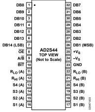
Figure 2. Pin Configuration
