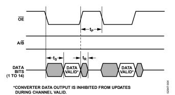
Figure 5. Alternative Reading of Each Channel
