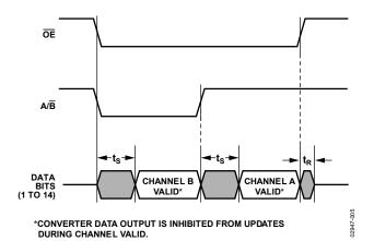
Figure 4. Repetitive Reading of One Channel
