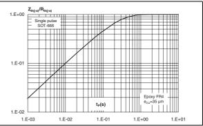
Figure 7. Relative variation of thermal impedance junction to ambient versus pulse duration (SOD-523)
