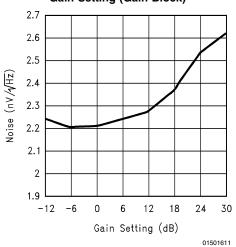
Noise Figure vs. Gain Setting
