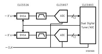
FIGURE 4. Diversity Receiver Chipset Block Diagram
