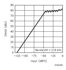
FIGURE 5. Diversity Receiver Chipset SINAD vs Input Power
