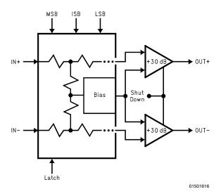
FIGURE 1. CLC5526 Block Diagram
